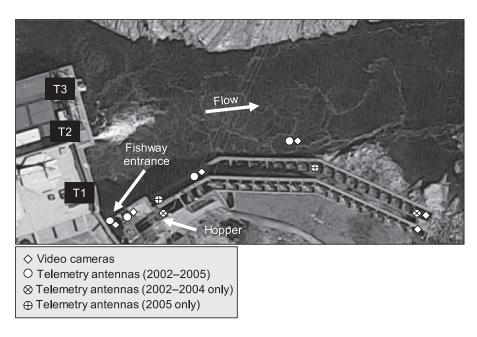
FIGURE 2. An aerial view of the Brunswick Dam (left) and fishway (bottom). T1, T2, and T3 denote the locations of the three hydropower turbine units. Areas where underwater video cameras were deployed are denoted by diamonds, and locations of telemetry receivers are represented by unique circle symbols denoted for specific years. Arrows depict the direction of flow and locations of the fishway entrance and hopper.
